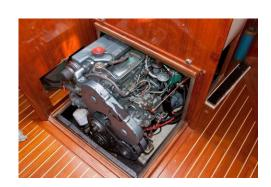
Changing diesel filters are another way in which oily contaminants can end up in the bilge – when switching these filters, make sure you do so over a container to catch any drips for safe disposal on land
